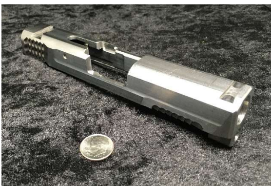
Figure 1- Actual Pistol Slide part machined on our HCN-4000 HMC
